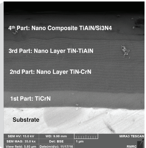
structure of Quad nano coating
