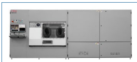
شکل ۵. LPCVD شرکت Equipment Corporation [۸]
